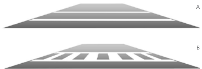
Crosswalk A is a traditional parallel line crosswalk. Crosswalk B is high-visibility crosswalk with a ladder design
